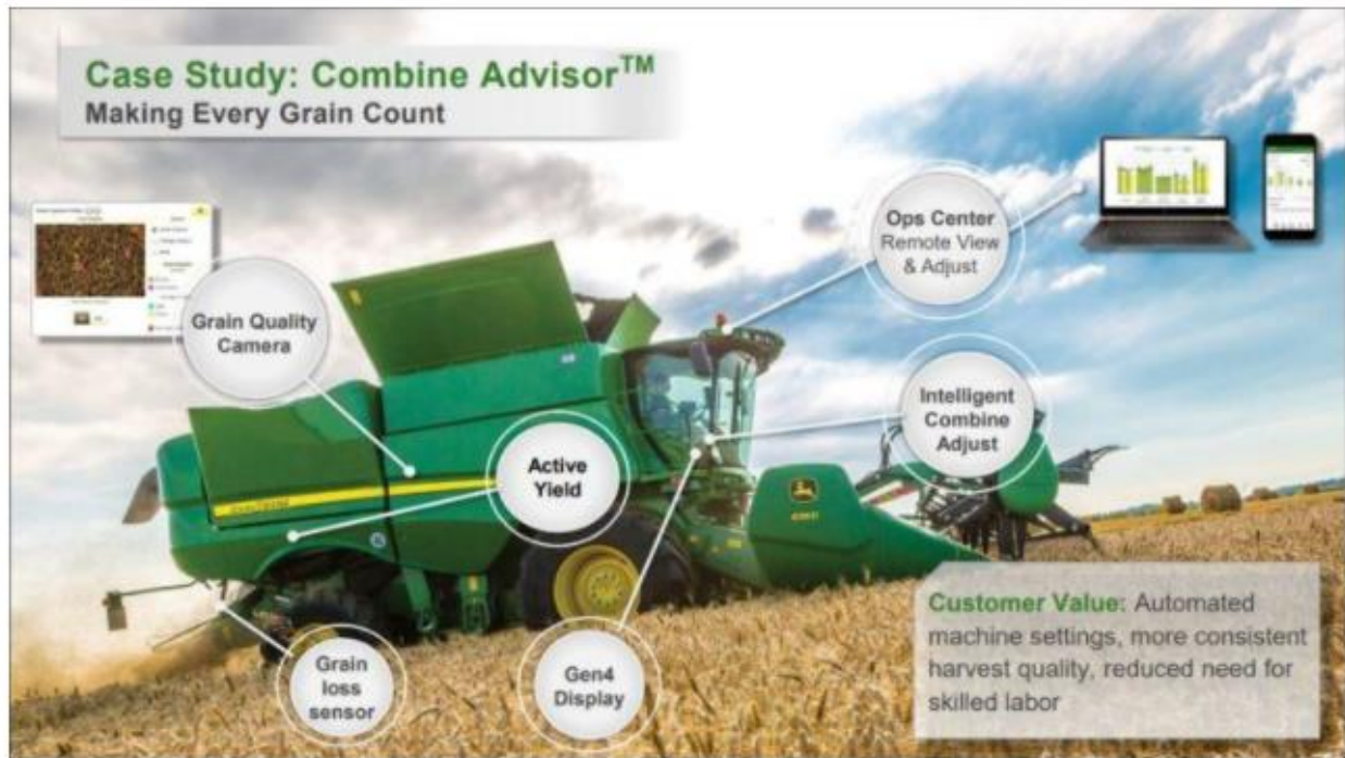
Figure :4.1. Example of combine that retrieves data through sensors and camera (Source: John Deere Investor Presentation August 2019)
