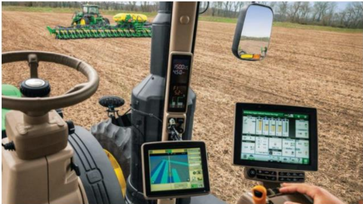
Figure 4.3. Maps showing machine field coverage reduces over-application of inputs, leading to lower input costs (Source: Deere.com)
